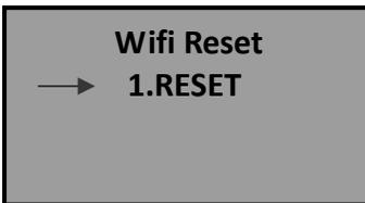
Short time button press move the cursor, and long time button press reset the wifi module.
